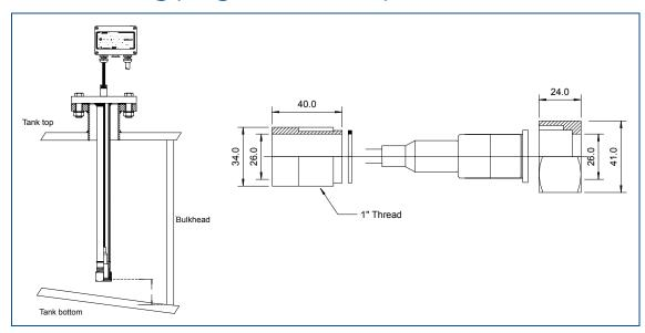
The weldable collar and the nut are manufactured of ASTM 316L steel. The gaskets are made of nitrile rubber.
